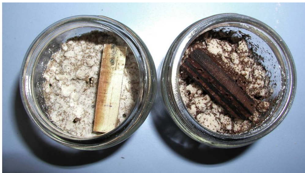
Fig. 6. Termite attack on untreated (on the left) and heat-treated wood (on the right). Adapted from Esteves (2006).
