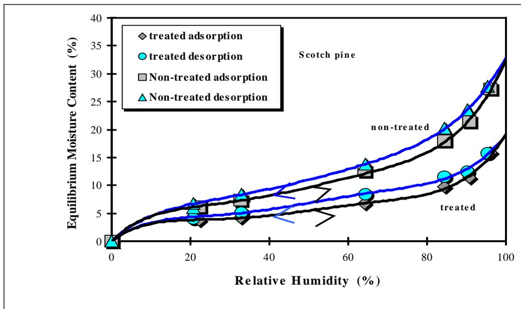
Figure 3: Hygroscopicity of treated (chemically or thermally) and untreated Scotch pine.
